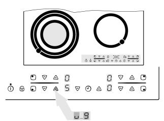
Touch the sensor field "triple ring zone" sensor field
